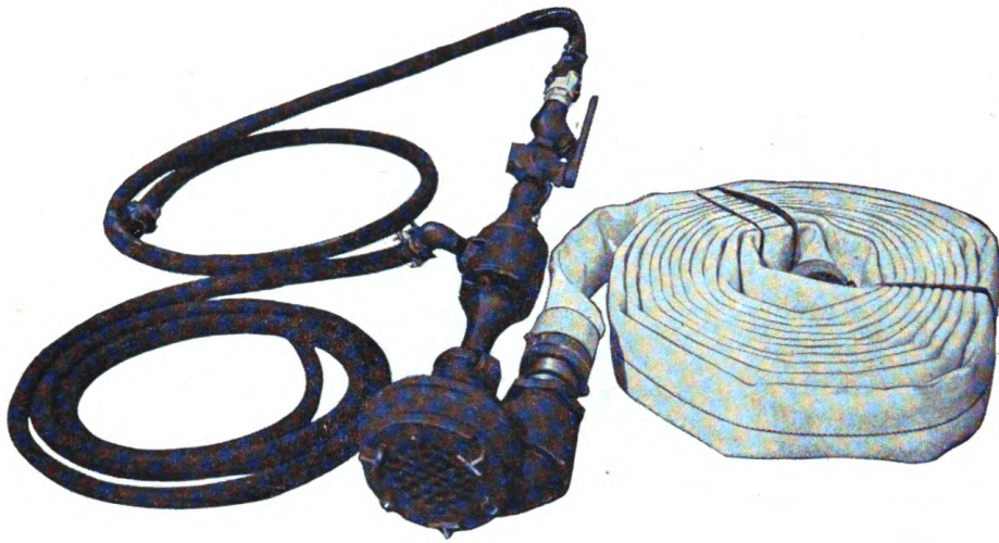
Figure 220. Pump, sump, pneumatic, 3-inch discharge, 175 gallons per minute, 25-foot head.
